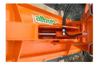
**Parking legs.** The snow plough is equipped with two parking legs. The parking leg should be in the retracted position when operating the snow plough. The parking leg can be extended and secured before detaching the snow plough from the telehandler. This allows the snow plough to be parked ready for use and simple reconnection.
