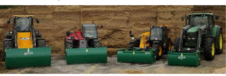
The shear grab blades must be checked and sharpened as required and at least once weekly using a file
