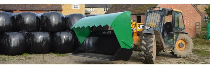
The shear grab blades must be checked and sharpened as required at least once weekly using a file
